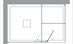
**B-6****Spessore 6 mm - PER INSTALLAZIONE SU PARETI IT-6, IT-8 E IT-C8****Thickness: 6 mm - FOR COMBINATION WITH PANELS IT-6, IT-8 AND IT-C8****misure standard Standard measures**
